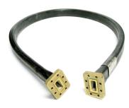
FlexTwist® Flexible Twist for WR28, 37.0–40.0 GHz, with interface types UG-599/U and PBR320, 900 mm
