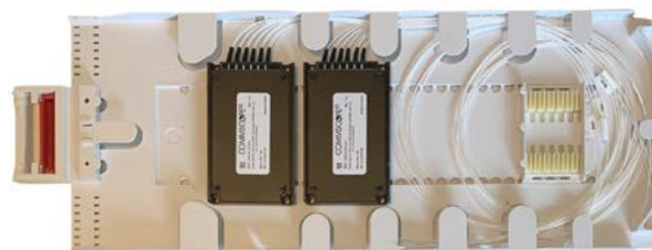
Example of S CASE installed onto FOSC D Tray
