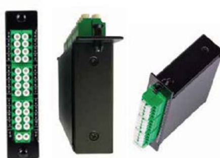
Single-width LGX module (4-, 8-, 10- and 20-channel configurations)
