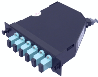
Fiber Optic MPO-LC Module, XG, 12 LC/UPC adapters, Singlemode fiber, blue
