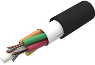
Fiber OSP cable, TeraSPEED® Mini Single Jacket, Gel-Filled, Outdoor Stranded Loose Tube, 48 fiber, Singlemode G.652.D and G.657.A1, Meters jacket marking, Black jacket color
