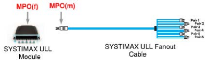
Figure 18. SYSTIMAX ULL MPO(m) fanout cable
