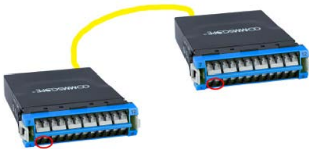
Figure 10. SYSTIMAX ULL module are orientated in the same direction at each end of the link
