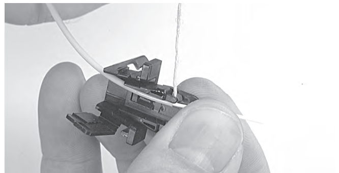
5.10 In case of less kevlar (typically this means pigtail diameter < 2,3 mm); wrap the kevlar to ensure a good strain relief.
