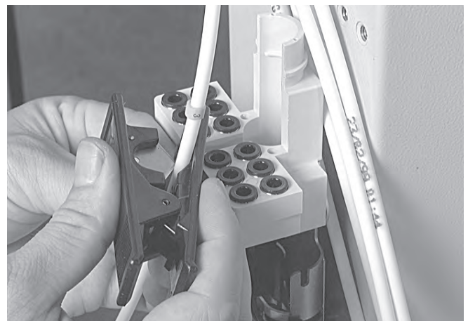
4.1.28 Cut the tubes to length using the tube cutter. Make sure the shelf is in an opened position.
