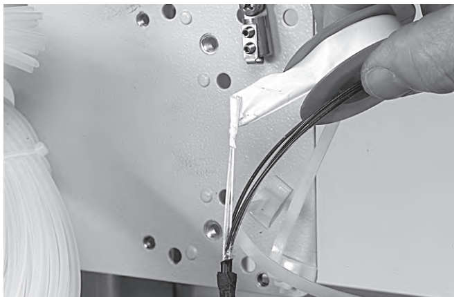
4.2.20 Wrap some layers of teflon tape around the ends of the strength members to keep them together.
