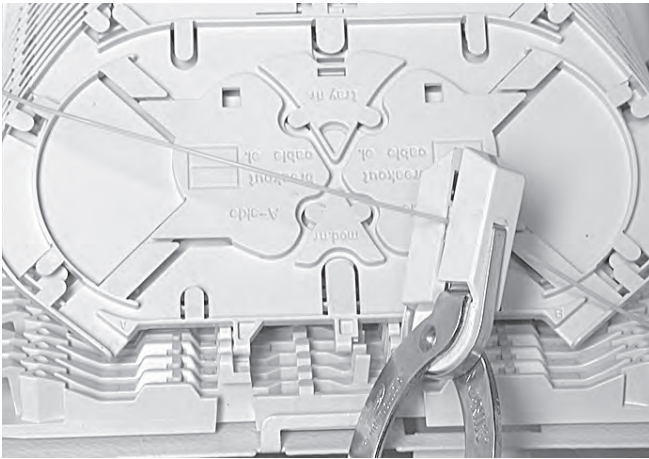
5.19 Make sure the transition of secondary to primary coating is in the splice protector. If this is not possible: strip the secondary coating (semi-tight) in the middle of the groove plate.
