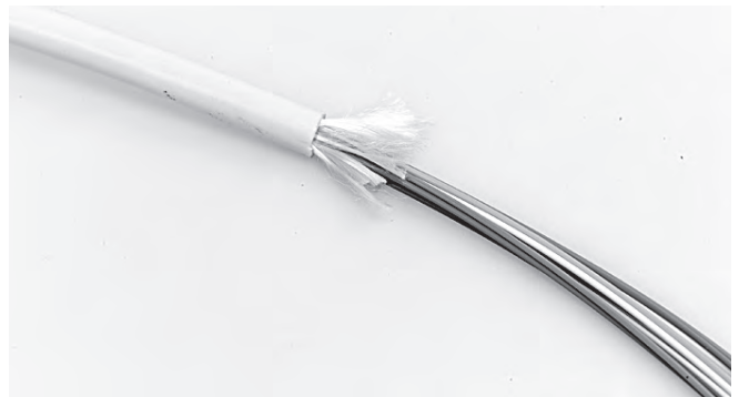
4.1.34 Remove the cable jacket over approximately 1.7 m.
