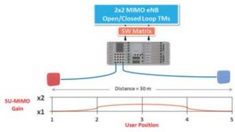
Figure 5: Interleaved single-user MIMO
