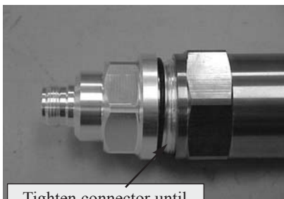
Tighten connector until O ring disappears.
