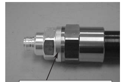
When properly tightened, there will be metal-to-metal contact here.
