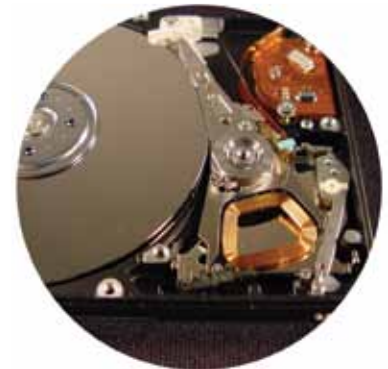
CCA used for computer hard drive
