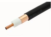
RCT6, RADIAX® Coaxial Radiating Cable with Bump, 50–2400 MHz, tuned foil, 1-1/4 in, black non-halogenated, fire retardant polyolefin jacket
