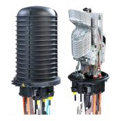
FIST® GCO2 Fiber Optic Splice Closure, Heat Shrink or Gold Gel Cable sealing, size BC, no pre-installed fiber trays, 16 round ports + 1 oval port with grounding, with test valve
