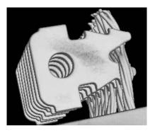
Figure 2 X-ray analysis of a terminated plug to stranded wires
