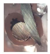
Figure 4 Micro-section showing typical contact interface achieved
