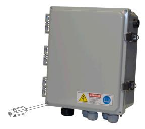
When assembly is completed tighten lid screws (qty 4) (0.6 N•m – 5 lb-in)
