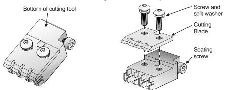
**Replacing Cutting Blade**
