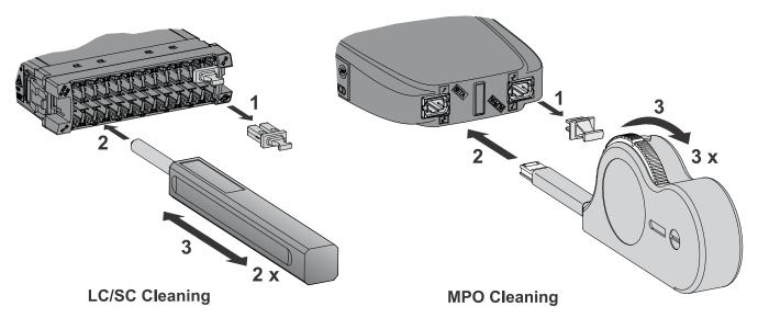
Clean each module port prior to installing a mating connector.
