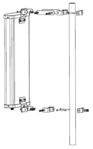
The antenna can be mounted to mounting hardware with a diameter of  $\Phi$  25 mm to 60 mm with supplied clamps.
