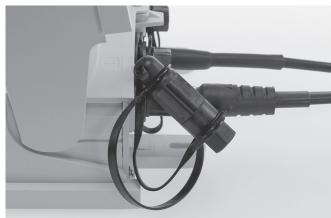
2.3 Connect the 2 dust caps from terminal port and hardened connector to keep the dust caps clean for future use.
