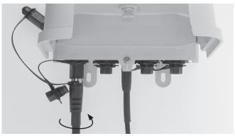
2.1 Unscrew the dust caps off both, the connector and the adapter, and install the hardened connector (hand tighten).
