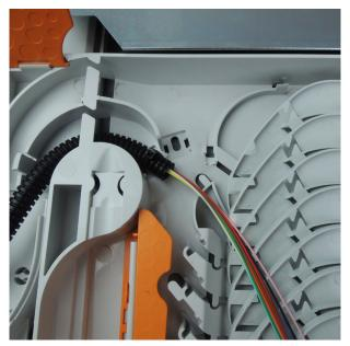
3.6 Fix the flex-tube with tie-wrap on splice drawer Repeat this steps for the second IFC-cable as well
