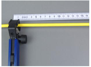
2.1.2 Cut the cable jacket at the marked point and approx. 150mm from the cable end to get access to the rip-cord
