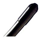
102K Heat-Shrinkable Cable End Cap kit, pressurized, for 16 to 26 mm cable diameter, 85 mm long, 600 pcs
