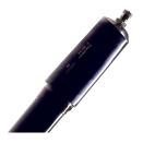
102K Heat-Shrinkable Cable End Cap kit, pressurized, with valve, for 71 to 90 mm cable diameter, 150 mm long, 70 pcs
