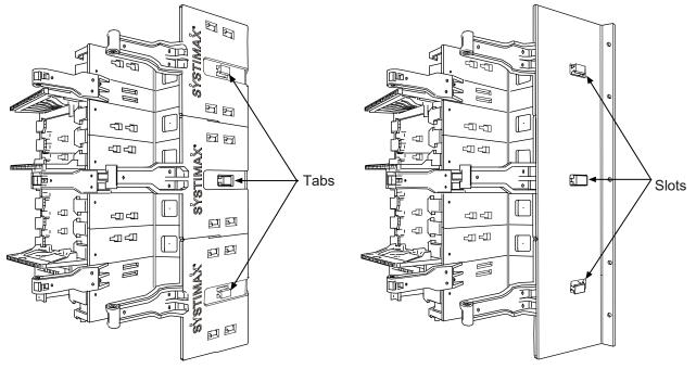
2. Locate tabs on outside of 12U vertical trough section per above figure. Position side panel as shown and hang it on side of vertical troughs so that tabs extend through slots in side panel per above figure.
