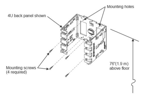
1. Measure 76 inches (1.9m) above floor and mark this position. Using a level, make additional alignment markings at this time to ensure the installation is level.
