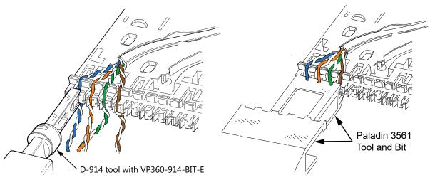
7. Using the D914 tool with VP360-914-BIT-E, seat and cut each pair of conductors. Be sure cutting edge is at the bottom.
