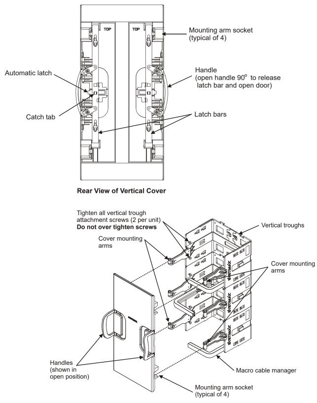
1. Open both handles on vertical trough cover 90° to set latch bars (see figure on top of previous page). An audible click will be heard when latch bars set. **Both handles must be opened and latch bars set before mounting covers.**
