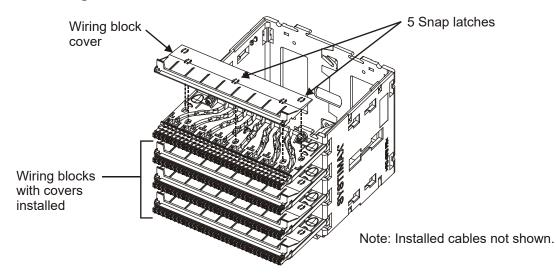
1. Position cover as shown above and push down onto wiring block until latches in cover engage in wiring block.
