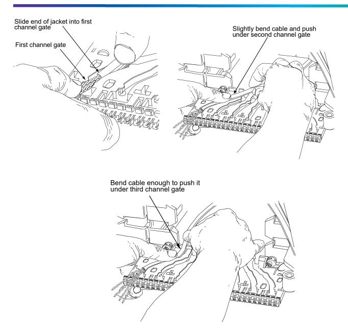
3. Seat each cable into one of the channels provided in wiring block as shown above. Insert cable so that end of jacket is under first gate in channel. Slightly bend cable and push into channel and under second gate. The cable should pop into the channel and catch under the gate. Continue inserting cable until it is seated under all three gates.
