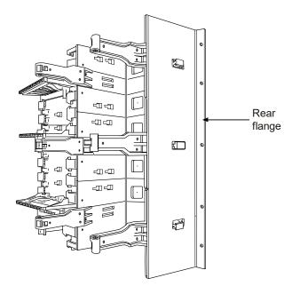
1. Remove one side panel from its packaging. Orient the side panel in relation to the vertical trough and wall surface as shown above for mounting on the right side.
