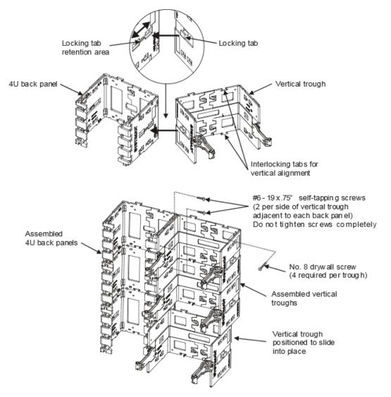
**Note:** Vertical troughs interlock with back panels on right and left sides.
