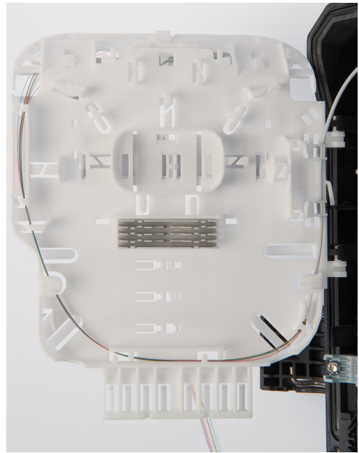
8.4 For splicing at the back of the tray, route the fibers as shown. Store fiber overlength in the top part of the organizer.
