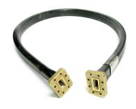
FlexTwist® Flexible Twist for WR28, 26.5–40.1 GHz, with interface types PBR320 and UBR320, 600 mm
