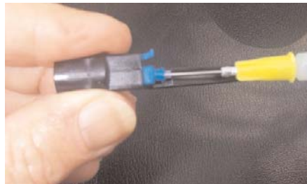
Inject adhesive into connector
