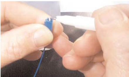
Scribe and cleave the fiber
