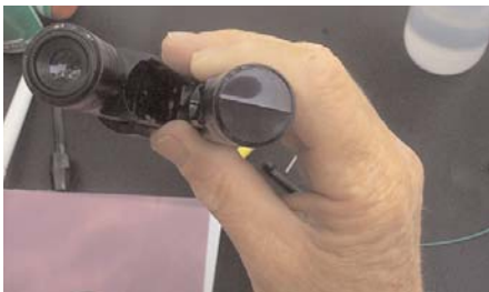
Inspect the connector face for any defects - be sure to clean prior to inspection
