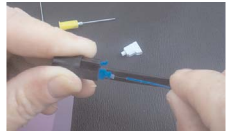
Insert fiber into the connector and allow adhesive to cure
