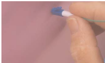
Air polish to remove the fiber stub
