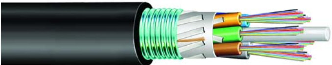
D-072-LA-XY-FZZNS All Dry Outside Plant Stranded Loose Tube Armored Cable
