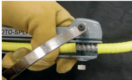
Step 14: Using the armor splitting tool, place the cable in the cable guide, tighten the thumbscrew and rotate the handle until the armor is cut. The armor splitting tool is designed to cut through with only one revolution of the cutter to protect the fiber cable inside.
