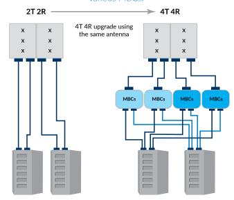
When combining multiple radios onto one RF path, there is an opportunity for unwanted passive intermodulation (PIM) interference. Therefore, operators should deploy only best-in-class, factory-tested, low-PIM MBCs.
