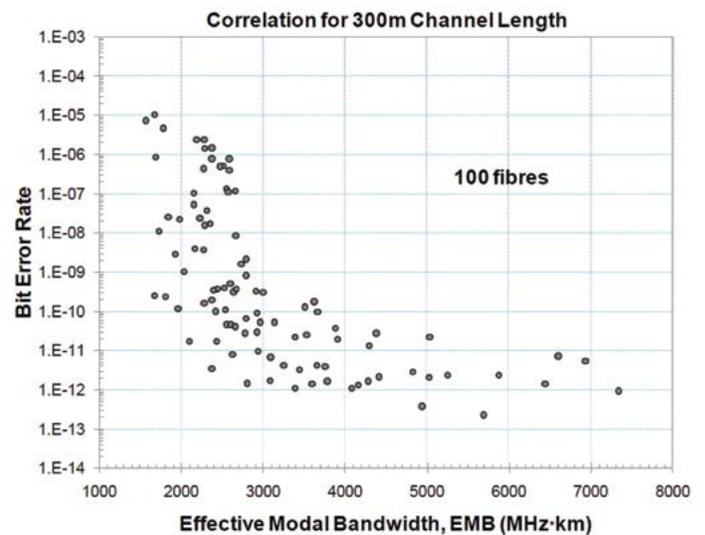
Figure 2. Bit error rate at -11.0dBm receive power for 100 fibers versus fiber effective modal bandwidth. The data shows poor correlation.
