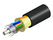
Fiber Indoor/Outdoor cable, TeraSPEED® Low Smoke Zero Halogen Riser Distribution, 24 fiber single-unit, Gel-free, Singlemode + Multimode OM1, Feet jacket marking, Black jacket color, Dca flame rating
