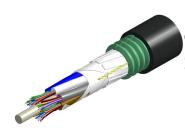
Fiber indoor/outdoor cable, TeraSPEED®, Single Jacket/Single Armor, 90 min Fire Survival, Low Smoke Zero Halogen (LSZH), 72 fiber, Singlemode G.652.D and G.657.A1, Gel-Filled, Stranded Loose Tube, Black jacket color, Meters cable marking
