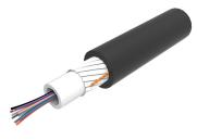
Indoor/Outdoor Low Smoke Zero Halogen, TeraSPEED® Central Loose Tube Fiber Optic Cable, 8-fiber, Singlemode OS2, Gel-filled, black. Provides Rodent Resistance.
