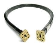
FlexTwist® Flexible Twist for WR90, 8.2–12.4 GHz, with interface types CPR90G and UBR100, 1200 mm
