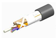
Fiber indoor/outdoor cable, TeraSPEED®, Single Jacket All-Dielectric, Plenum Rated, 48 fiber, Singlemode G.652.D and G.657.A1, Gel-Free, Stranded Loose Tube, PVDF jacket, Black jacket color, Feet cable marking
