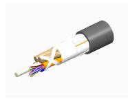
Fiber indoor/outdoor cable, LazrSPEED®, Single Jacket All-Dielectric, Plenum Rated, Gel-Free, Stranded Loose Tube, PVDF jacket, 96 fiber, Multimode OM3, Black jacket color, Feet cable marking
