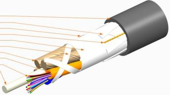
Plenum-Rated Outer Jacket Strength Elements Binder Water Swellable Tape Ripcord (1) Binder 2.5 mm Gel-Free Buffer Tubes 250 micron Fibers Dielectric Strength Member
