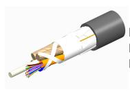
Fiber indoor/outdoor cable, LazrSPEED®, Single Jacket All-Dielectric, Plenum Rated, Multimode OM4, Gel-Free, 24 fiber, Stranded Loose Tube, PVDF jacket, Black jacket color, Feet cable marking
