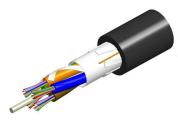
Fiber indoor/outdoor cable, TeraSPEED® Light Duty, Single Jacket, Riser Rated, 24 fiber, Singlemode G.652.D and G.657.A1, Gel-Free, All-Dielectric Outdoor Stranded Loose Tube, Black jacket color, Feet cable marking
