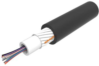
Indoor/Outdoor Low Smoke Zero Halogen, TeraSPEED® Central Loose Tube Fiber Optic Cable, 4-fiber, Singlemode OS2, Gel-filled, black. Provides Rodent Resistance.
