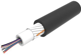
Indoor/Outdoor Low Smoke Zero Halogen, TeraSPEED® Central Loose Tube Fiber Optic Cable, 24-fiber, Singlemode OS2, Gel-filled, black. Provides Rodent Resistance.
