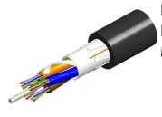
Fiber indoor/outdoor cable, LazrSPEED®, Light Duty, Single Jacket, Riser Rated, Gel-Free, All-Dielectric Outdoor Stranded Loose Tube, 2 fiber, Multimode OM3, Gel-free, Feet jacket marking, Black jacket color
