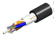
Fiber indoor/outdoor cable, LazrSPEED®, Light Duty, Single Jacket, Riser Rated, Gel-Free, , 12 fiberAll-Dielectric Outdoor Stranded Loose Tube, Multimode OM3, Gel-free, Feet jacket marking, Black jacket color
