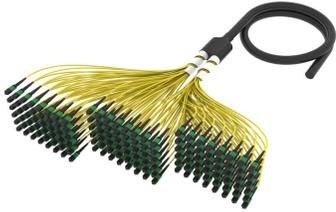
Ultra Low Loss ULL TeraSPEED® MPO (Unpinned) to Unconnectorized Pre-terminated Trunk Cable, MPO12, 1728-Fiber, LSZH/Riser, 12-fiber Rollable Ribbon I/O Central Tube
