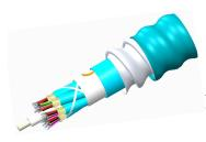
Fiber indoor cable, LazrSPEED® Riser/LSZH rated, Distribution, interlocking aluminum armored, Multimode OM3, 72 fiber multi-unit with 12 fiber subunits, Gel-free, Feet jacket marking, Aqua jacket color
