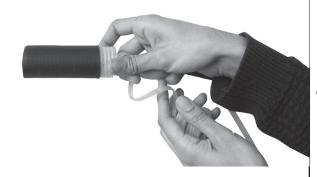
Plastic has been removed and is now even with the front edge of the shrink tube.
