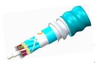
Fiber indoor cable, TeraSPEED® Low Smoke Zero Halogen Riser Distribution, interlocking aluminum armored, Multimode/Singlemode, 48 fiber multi-unit with 12 fiber subunits, Gel-free, Feet jacket marking, Aqua jacket color
