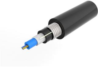
Fiber Indoor/Outdoor cable, TeraSPEED®, 120 min Fire Survival, Low Smoke Zero Halogen (LSZH), 6 fiber, Gel-Filled, Central Loose Tube, Singlemode G.652.D and G.657.A1, Meters jacket marking, Black jacket color. Provides Rodent Resistance.
