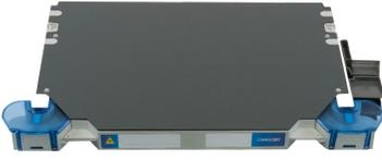
FACT® Fiber Optic High Density Patch Chassis, gray, 1E high, 72-port, singlemode, holding 2 hinged trays loaded with LC adapterpacks to be used with 1.2 mm simplex patch cords
