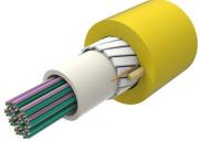
Fiber indoor cable, Riser All-Dielectric Central Tube, 16-fiber Rollable Ribbons, 288 fiber, 200um Singlemode G.657.A2, Feet jacket marking, Yellow jacket color
