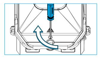
1 Secure by turning the locking screw.
