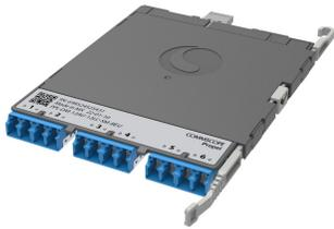
Propel ULL Singlemode MPO-12 Distribution Module, 6 duplex LC/UPC to 1X12f MPO/APC pinned, Method B Enhanced
